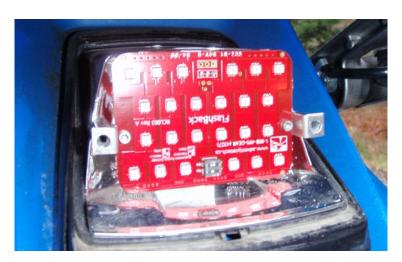
**Note:** For bikes that require you to screw mounting brackets into taillight reflective housing we have supplied 2 machine screws in a zip lock bag for you. They require a Phillips screwdriver. It is important that when aligning the board it is not tilted up or down as this will affect the visibility of the light. Once screws are in place recheck
